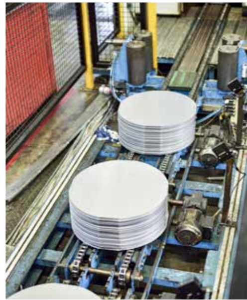
Unloading a coil (top left) and lifting it directly into one of the two coil warehouses by crane. The narrower plate used to press the rims is loaded onto the reel in the cut-to-length line (left), while the wider plate is pressed into blanks for wheel disc production by the cutting press (right). All production processes are highly automated and are both controlled and monitored by computers (below)
