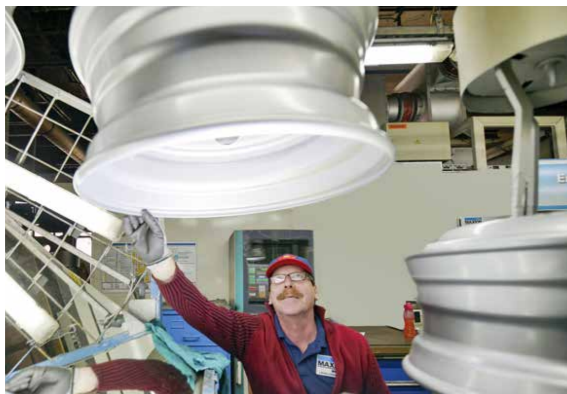
A final check in the paint shop: A team member examines the silver or black wheels under neon light
